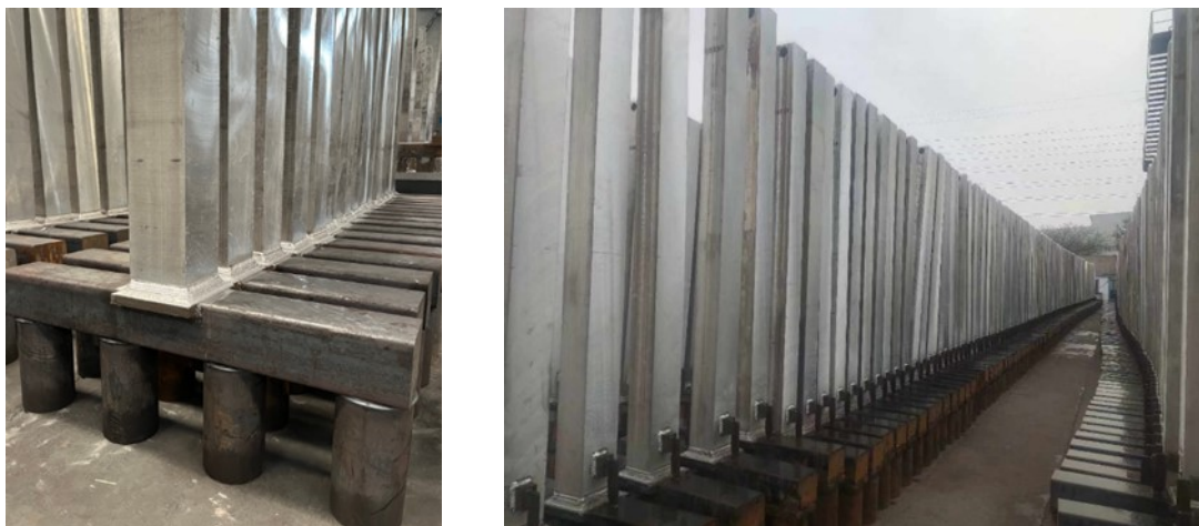
Figure 11. Industrial application of direct welding technology for steel and aluminium.
