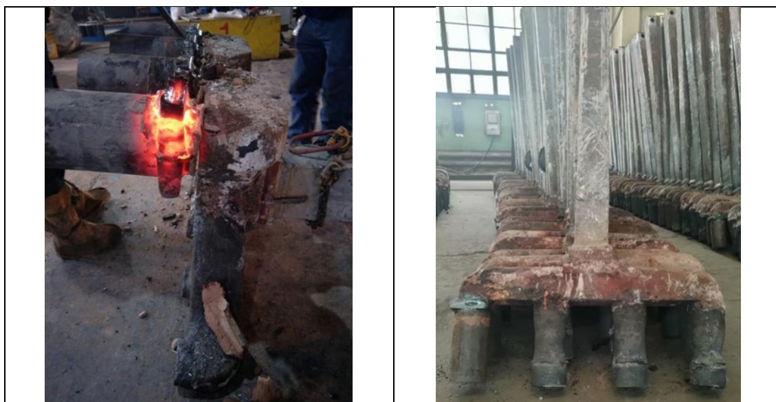
Figure 13. Industrial application of narrow-gap full-section welding of anode steel stubs.
